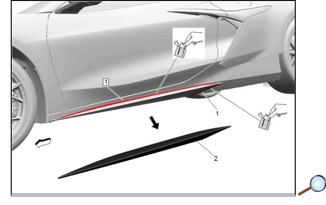
6. Test fit rocker panel molding (2) in position. Note the area of attachment tape contact (1) and remove rocker molding (2). Clean the area with the solvent wipe.
