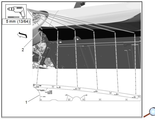
**Caution:** Always check scale, size and position of all templates before drilling. Failing to do so may cause damage to the vehicle, misalignment of components or the inability to install the accessory.
