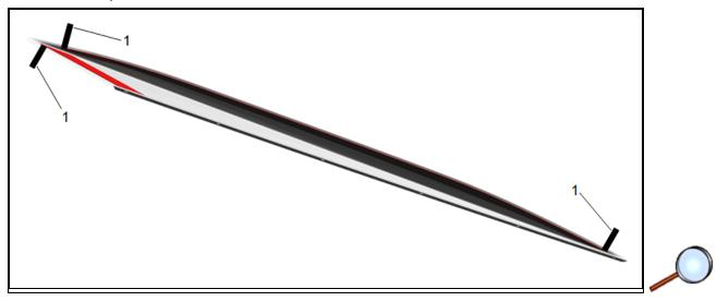
7. Using masking tape, secure the attachment tape release tabs (1) so they can be accessed after the molding is installed.
